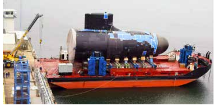
The bow section of the Virginia-class attack submarine USS North Dakota arrives in December 2012 at General Dynamics Electric Boat in Groton, Conn., after being barged north from the Newport News Shipbuilding submarine plant. (General Dynamics Electric Boat file media photo by Robert Gallo published by the Associated Press.)
