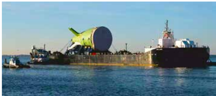
The stern section of a Columbia-class ballistic missile submarine in June 2024, while en route from Virginia's Newport News Shipbuilding to General Dynamics Electric Boat in Groton, Connecticut. (File media photo via Huntington Ingalls Industries.)
